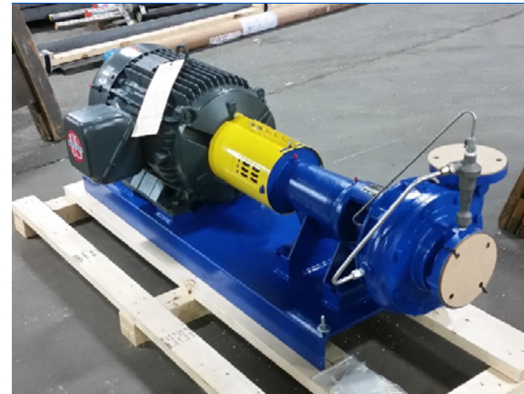
40HP 3x2.5x10 Frame-mounted GH with plan 31 Cyclone separator
