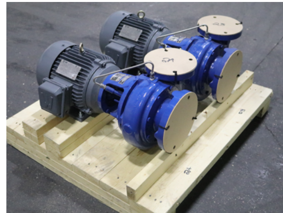
3HP 4x3x7 Close-Coupled GH with plan 11 seal flush and motor space heaters
