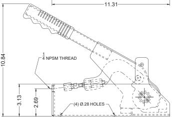
Betts Deluxe Mechanical operators function cable operated emergency valves from a central location on a cargo tank. Operators are available in any number of compartments from 1 up to 5. Each compartment is supplied with a fusible joint designed to melt at not more than 250° F. Non-slip cable connectors for each compartment allow cables to be cut to length after installation.
